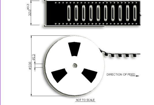
Tape and reel conform to IEC 60286-3 standards 40-80 g pull-force will be required to peel cover-tape 2000 sensors will be packed in one reel
